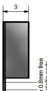
The component must be coated on the board to prevent electrical arcs
