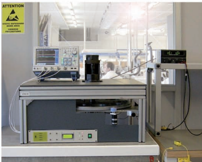
Custom made Jig for optical encoders dynamic tests.
